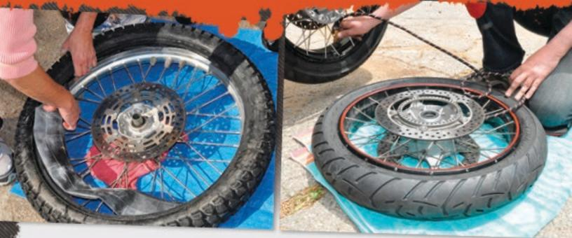
**Left** When feeding a tube back into its tire, start by inserting the valve stem. Screw the locking nut on so that it barely clears the top of the stem. The valve stem should move easily up and down within its exit point on the rim. The nut will be tightened down at a later step in this process.
