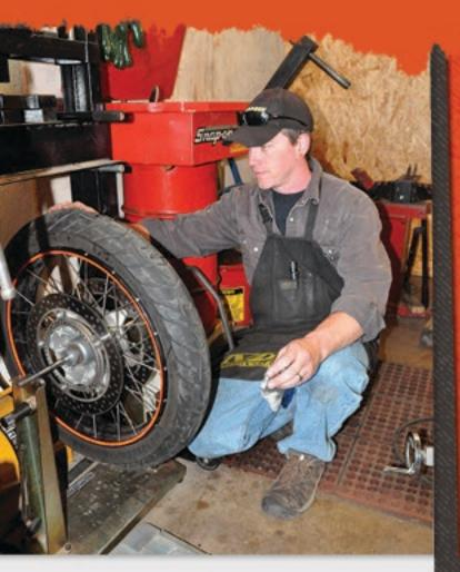
Traditional lead weight wheel balancing being performed by Curtis Smith of Eurogeek Motosport, in Flagstaff, AZ. While learning about Dyna Bead techniques, I was forced to resort to the traditional default method. The culprit turned out to be not using enough Dyna Beads to do the job correctly.
