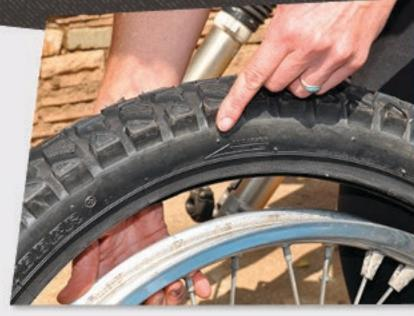
Most tires have a direction of rotation indicator imprinted on one of the sidewalls, normally in the form of an arrow. Few things are more infuriating than discovering you forgot to pay attention to the arrow until after the tire has been mounted.
