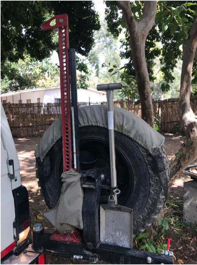
Spade and High lift jack mounted custom on dual wheel carrier
