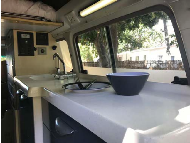
Sink and workspace in kitchen, hot/cold water tap and waterfilter tap. Geyser 15 liter, runs on DC or gas. 60 or 70o water temperature. Hot water in 10 minutes, also to use for outdoor shower.
